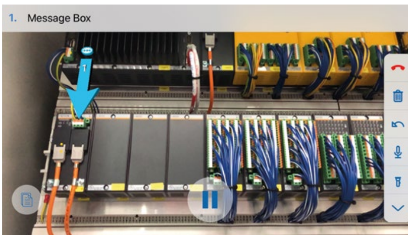
Fig. 4 Dorst remote service support using augmented reality glasses
