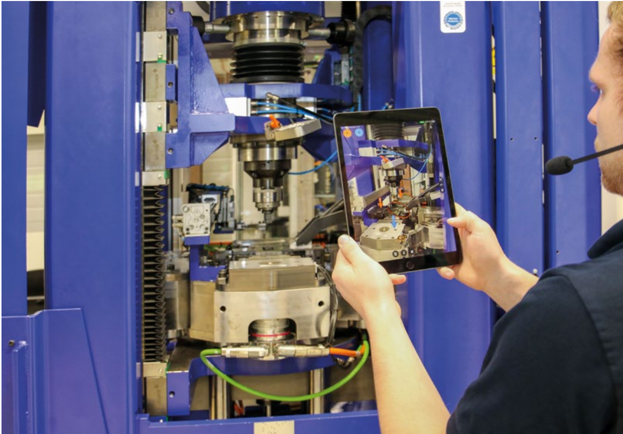
Fig. 5 Dorst remote service support using smart devices
