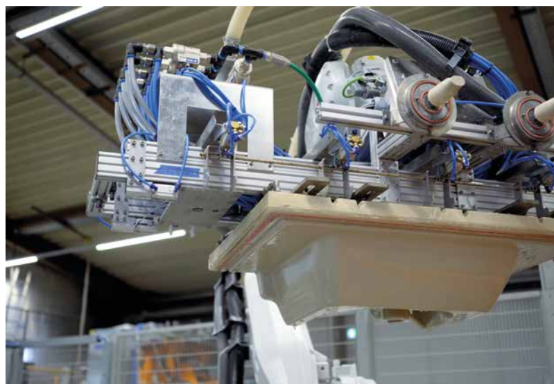
Fig. 3 Robot unit of the production system during demoulding of an article from the DORST COMPACTCAST 300
