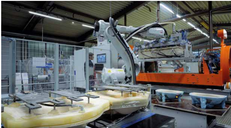
Fig. 4 Robot unit of the production system during mould change on the DORST COMPACTCAST 300
